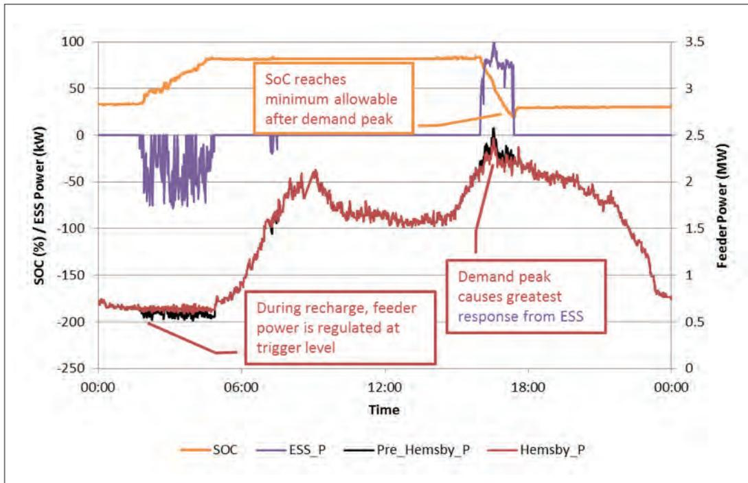
Figure 1 - Results from one day of peak shaving (load shifting)
