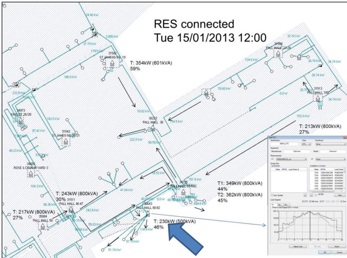
Figure 1. Potential transfer profile of a RES (Pall Mall 80-82)
