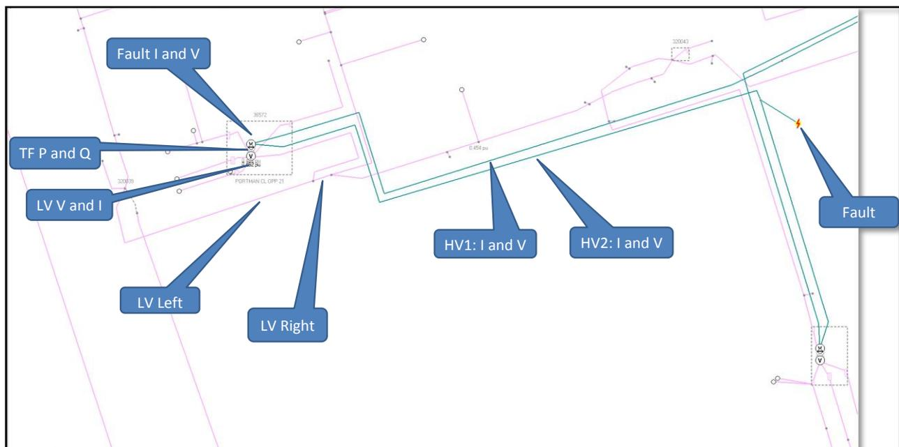
Figure 7. Validation of Reverse Power fault current flows in DPlan
