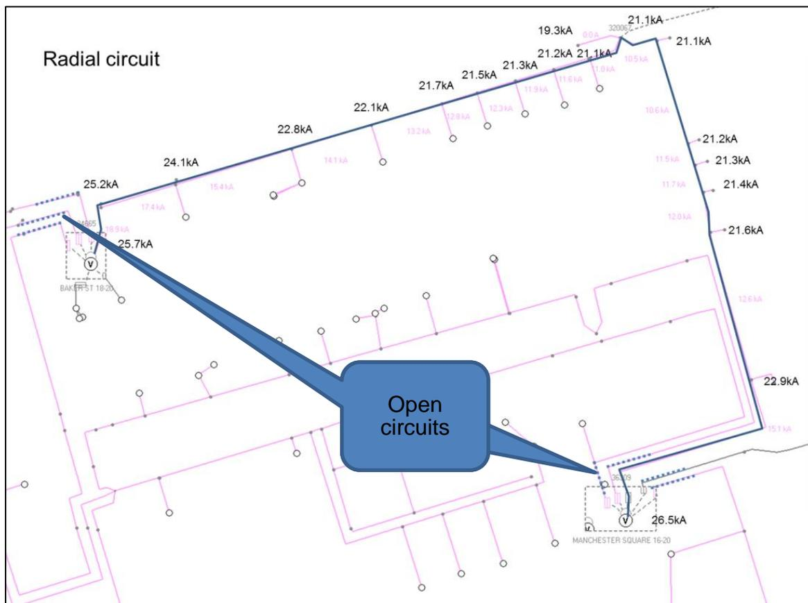
Figure 9. Example of DPlan used for studies for how radial circuits perform when they are meshed
