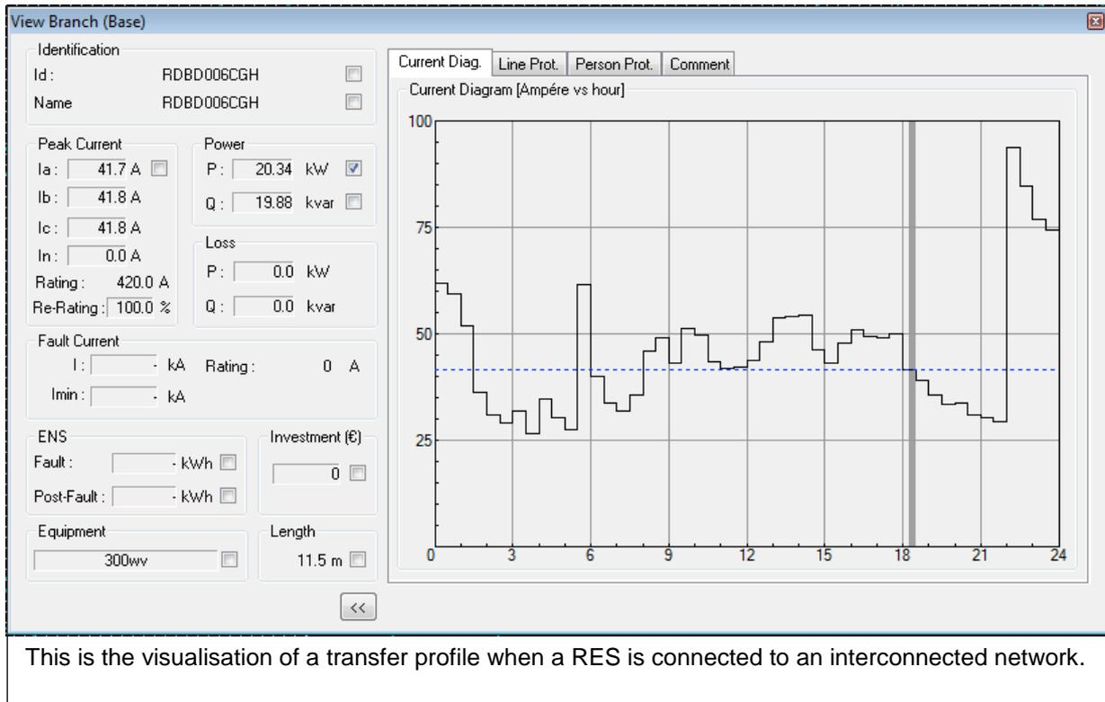
Figure 2. Visualisation of transfer profile for a RES using load flows capabilities in DPlan
