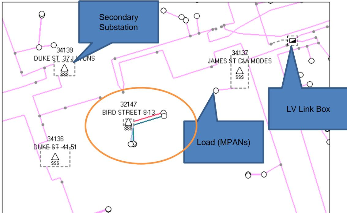
Figure 4. DPlan representation of substations and feeders
