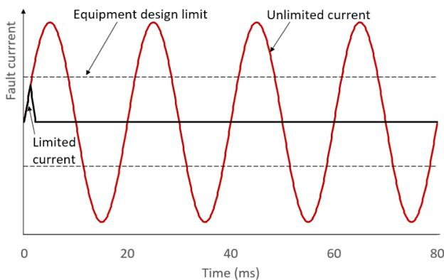
Figure 3. Fault current limitation using a hybrid FLCB.
