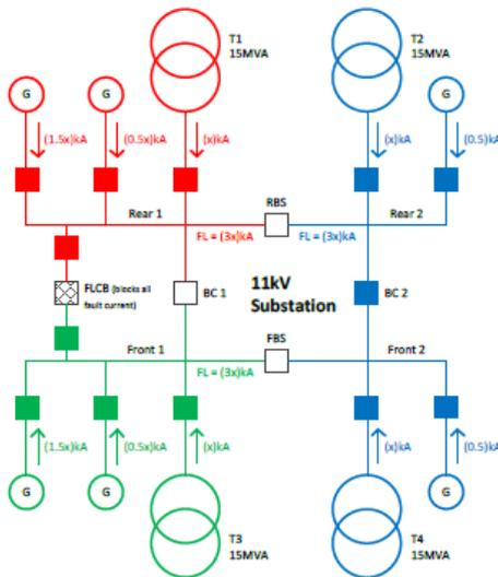
Figure 6. FLCB introduced as a bus coupler.
