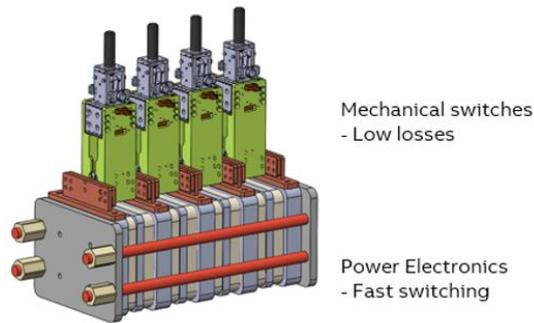
Figure 9. Modular concept of the FLCB for UKPN.
