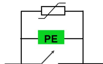
Figure 1. Principle of the hybrid fault current limiter.
