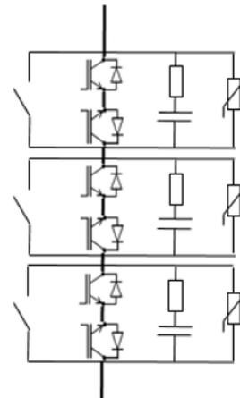
Figure 8. Modular concept of the FLCB for UKPN.
