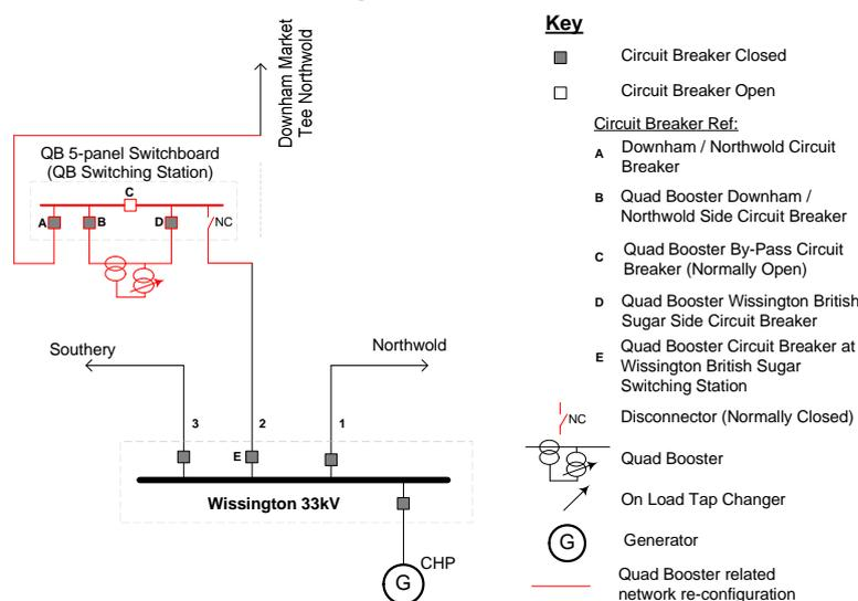
Figure 2: Simplified Single Line Diagram
