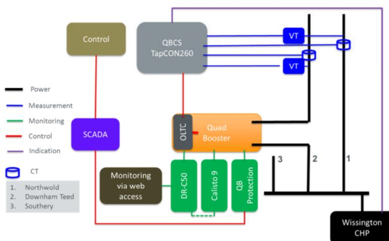
**Figure 3: Simplified Quadrature Booster architecture**
