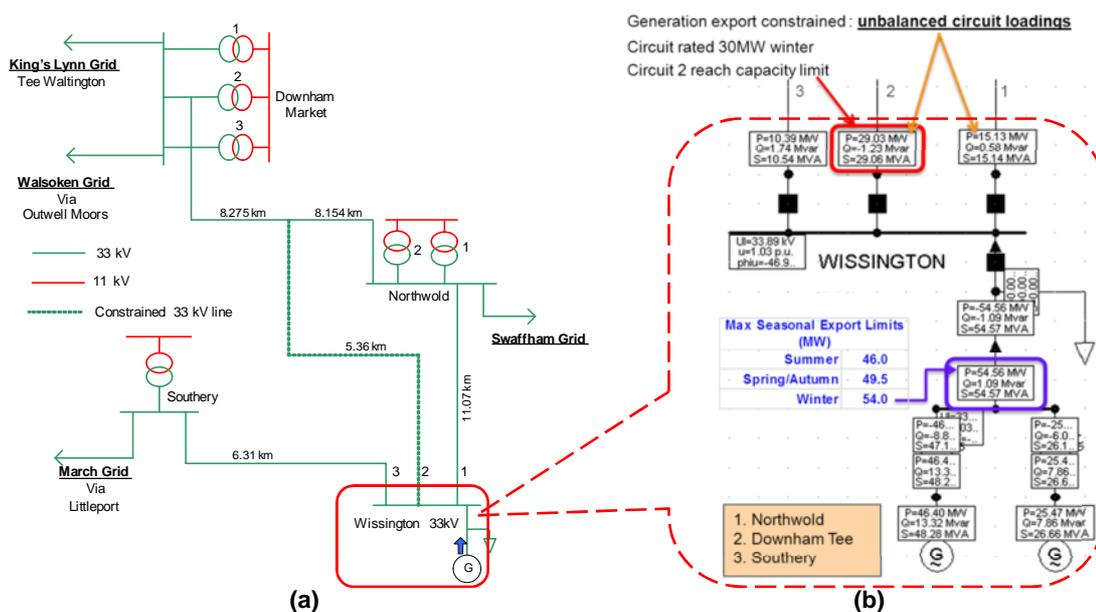
Figure 1: (a) Simplified Wissington 33kV Network, and (b) related Load Flow indications
