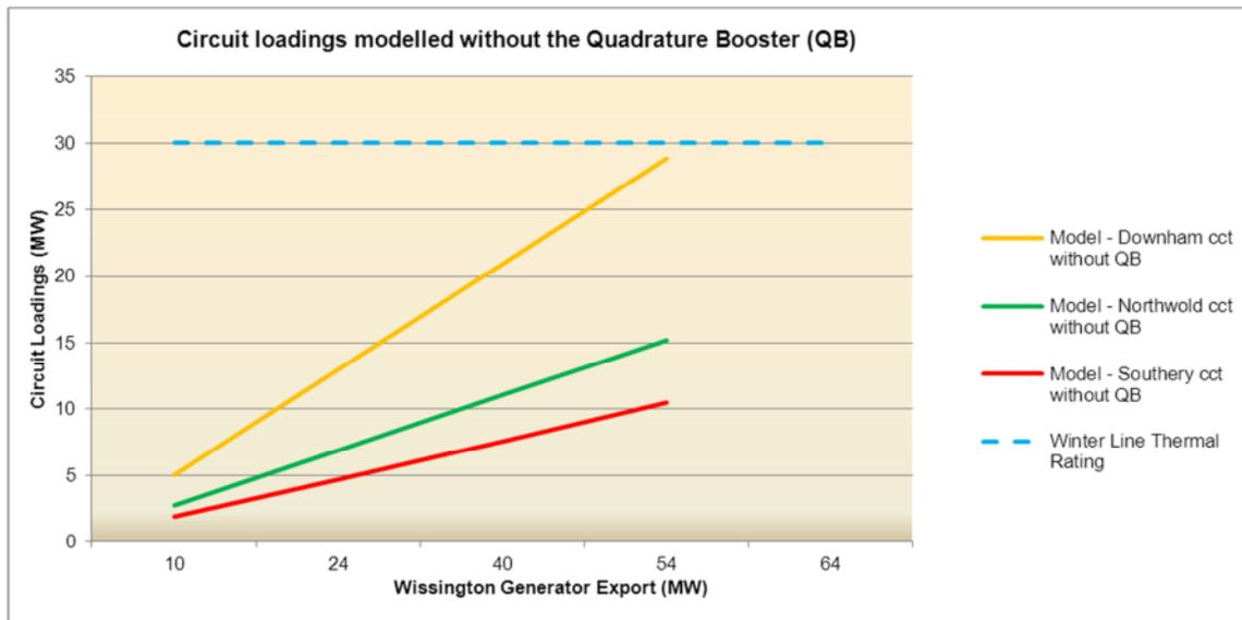
Figure 6: Modelled circuit loadings without Quadrature Booster
