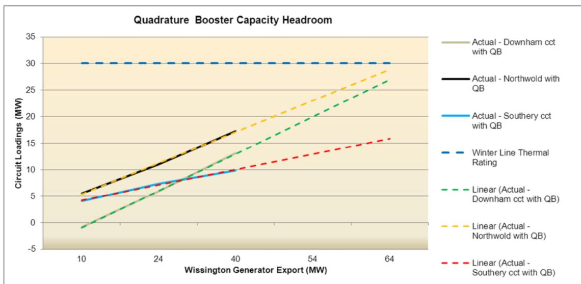
Figure 7: Graphs showing measured line loadings - and extrapolations
