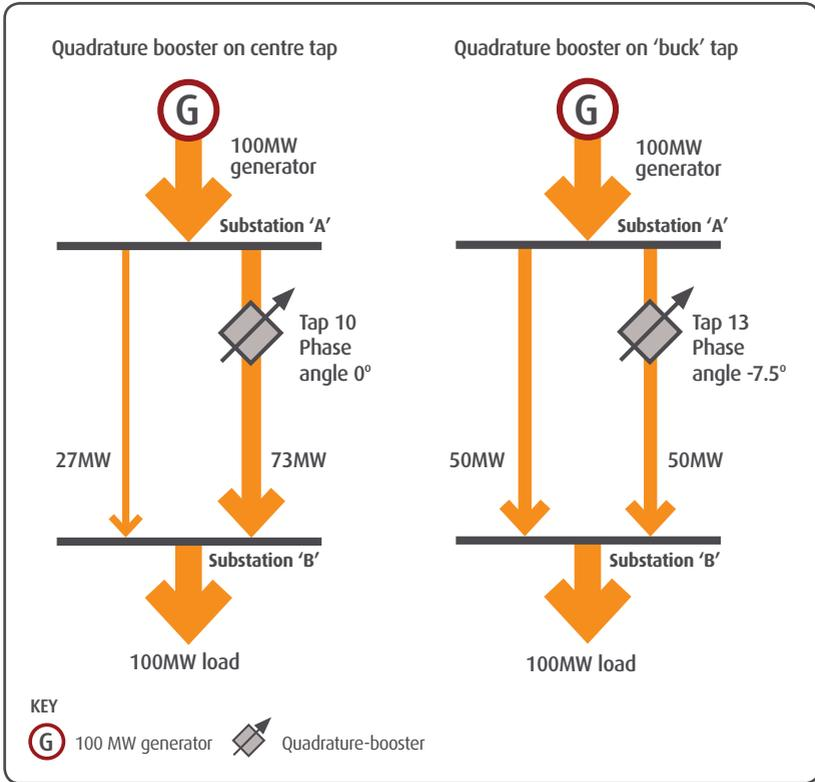
The diagram above illustrates how a Quadrature-booster works. On the left the Quadrature-booster is shown on 'centre tap', the lines out of balance - one line has 73MW and the other has 27MW. On the right the Quadrature-booster control system
