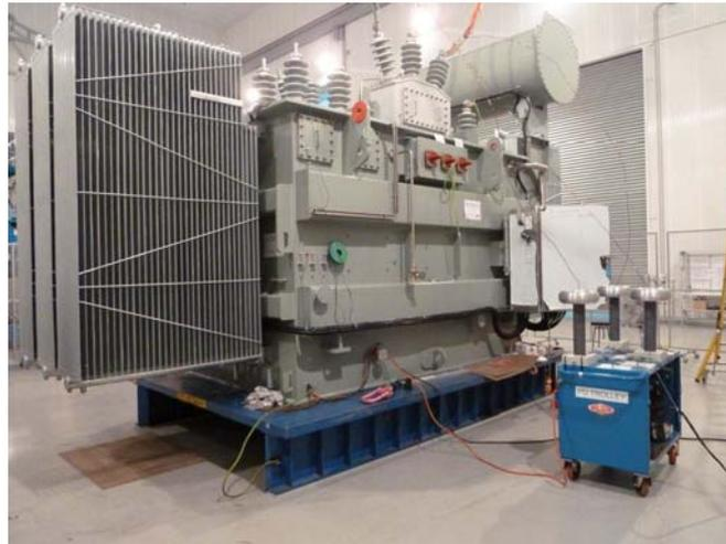
**Figure 2: General view of Quadrature-Booster in test at the factory (January 2013)**
