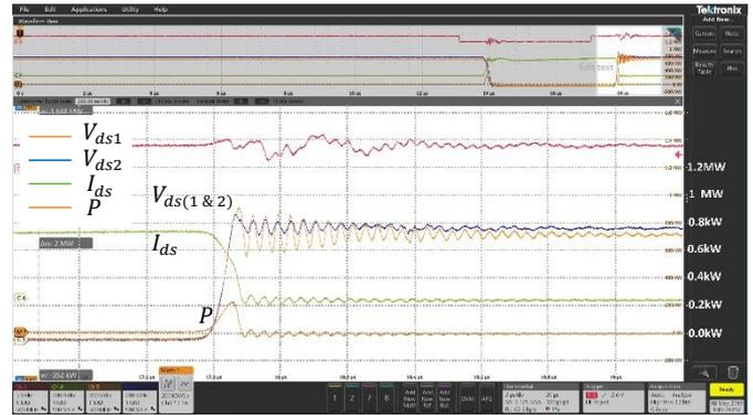
Fig. 11 Switching power losses with Snubber. Ch5 –  $V_{ds1}$  200V/div, Ch6 -  $V_{ds2}$  200V/div, Ch4 - Device Current  $I_{ds}$  200A/div, Time 200ns/div
